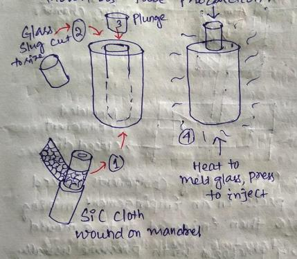
Ly A preform & a glass slug. are Enterested Ento a cylindrical mould. Application of heat & press. forces the fluid glass Ento the pores in the preformed after cooling the composite tube is ejecto from the mould.
