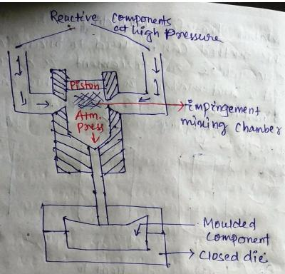
Here two fast reacting components mixed at high press. En an Empingement mixing Chamber & then Enjected in to a mould containing preform with pressure usually less than 1 Mps. This is followed by rapid curing so the cycle time for this process which is known as reinforced reaction Enjection moulding (RRIM)
