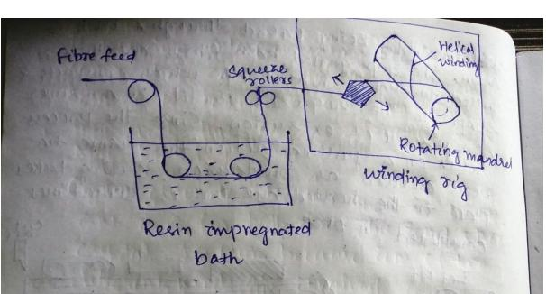
1) Filament wound components include pipewong pressure vessels, storage tanks & aerospace Parts Such as helicopter blades.
